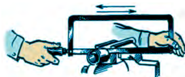
60-rasm. Trubalarni chilangarlik arrasi bilan qirqish.
