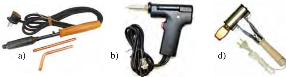
77-rasm. Kavsharlagichlar: a – oddiy; b – to‘pponchasimon; d – bolg‘asimon.
