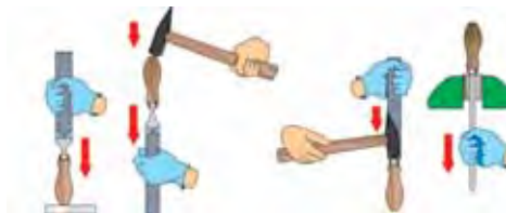
13-rasm. Egov dastasini qotirish usullari.
