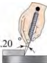
46-rasm. Chizma bo‘yicha to‘g‘ri burchakli detallarni rejalash.
